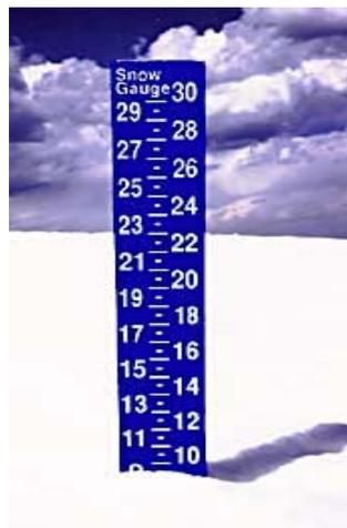
A snow gauge is a very simple, inexpensive device that measures snowfall accumulation. It has spring steel legs which allow it to withstand strong winds and the numbers are large enough that it can be read at a distance (from indoors).
