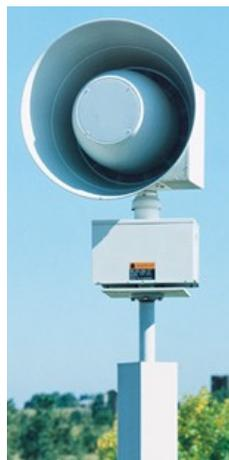
Electromechanical sirens emit a very powerful sound in all directions due to a rotating head. This particular model has a sound output of 128dBC and has an effective range of 5,600 feet. Most electromechanical sirens run on AC power but some models are available that can use rechargeable batteries, or even solar power.
