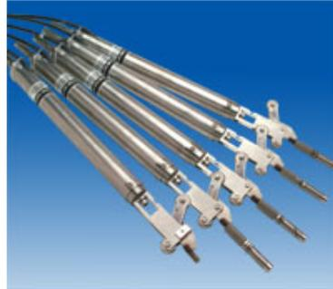
An inclinometer is a device used to monitor slopes and landslides. It can detect whether movement is constant, accelerating, or responding to any mitigation measures. A series of fixed sensors (shown above) can be implanted into the hazardous region. The sensors measure a change in inclination and can trigger an alarm when a preset inclination value, or rate of change value, is exceeded.
