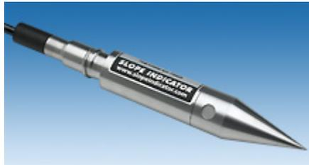
A Piezometer is used to measure pore water pressure. This is useful in determining slope stability as an early indicator for a landslide. The vibrating wire piezometer converts water pressure to a frequency via a diaphragm, a tensioned steel wire, and an electromagnetic coil. The piezometer is also equipped to measure temperature. The signal can be transmitted great distances with a properly shielded cable.
