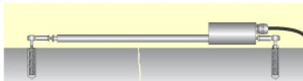
A crackmeter is a device that can be used to monitor movement over a crack in the rock. The ends of the device are anchored in the rock and a transducer is mounted across the anchors. If the distance across the crack changes, a signal is produced which is recorded by a data logger.
